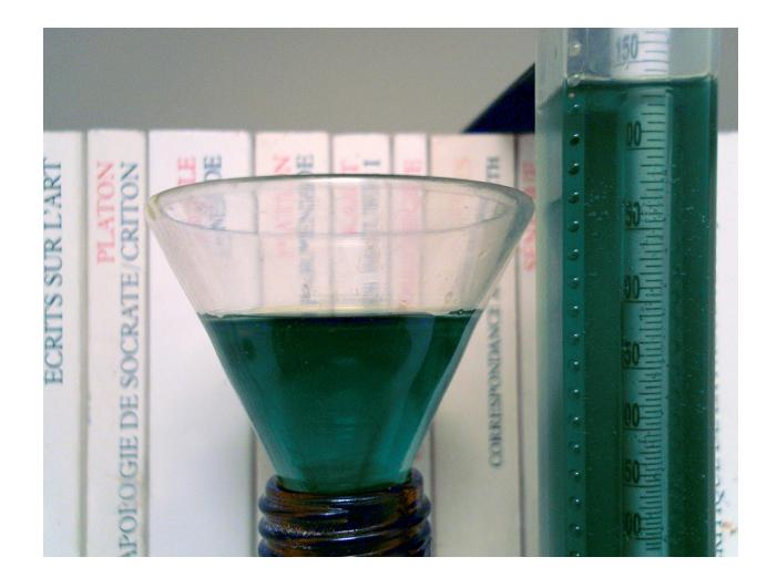
The simplest way of measuring this concentration is to use an aerometer as shown above.
