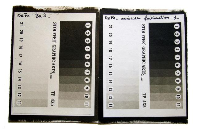
We can notice on this image that the gradation is approximately the same, on the other hand the density of the blacks shows big differences that we can measure with a densitometer, even if on the print above this difference is not visible.
